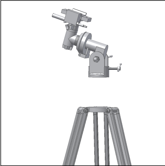
Figure 4. Place equatorial head on top of tripod.
