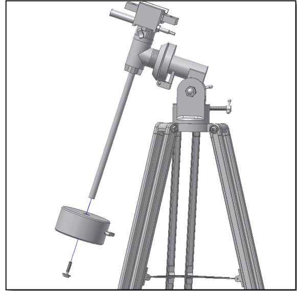
Figure 5. Thread the counter-weight shaft. Insert counterweight.
