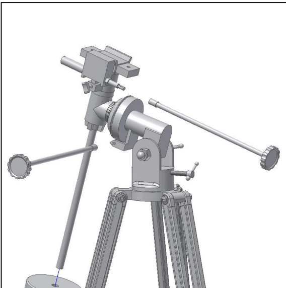
Figure 6. Fix Dec. and R.A. handles.
